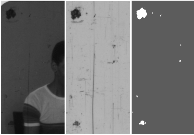
(a) Y component (b) Objective GT (c) dirt mask of GT Fig. 10. (a) luminance component of original frame, (b) corresponding greylevel GT data and (c) binary GT mask obtained from (b).
