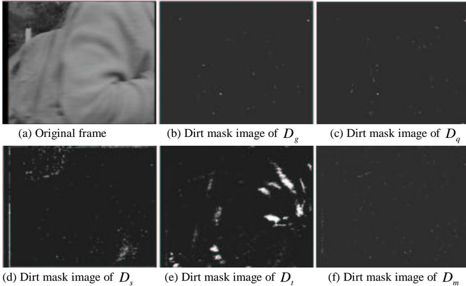
**Figure 10:** One test image and dirt mask images of ground truth ( $D_g$ ) and results from approaches of our method ( $D_q$ ) and spatial ( $D_s$ ), multistage ( $D_m$ ) and temporal ( $D_t$ ) median filtering.
