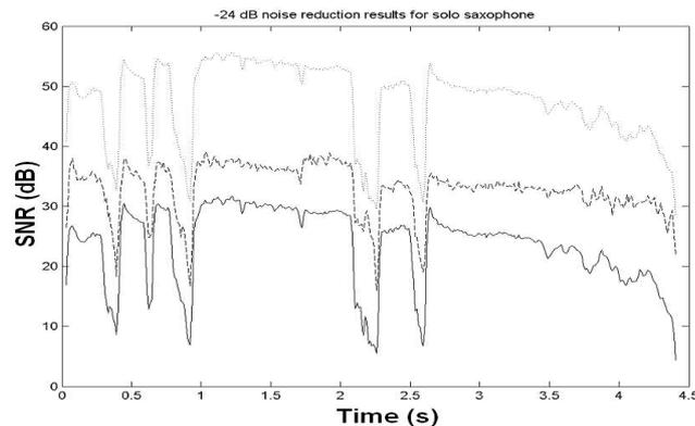
**Fig. 5.** Time varying SNR for 24 dB noise attenuation, calculated for each processing frame, for input signal (solid line), for perceptually reconstructed signal (dashed line) and for signal restored with spectral subtraction (dotted line), which was used as the *rough estimate* of the restored signal
