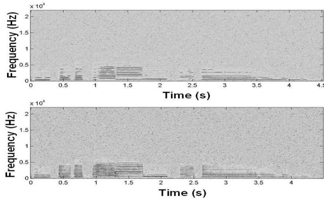
**Fig. 6.** Spectrograms of signal restored with spectral subtraction (upper plot), and with spectral subtraction enhanced by intelligent pattern recognition system (lower plot)
