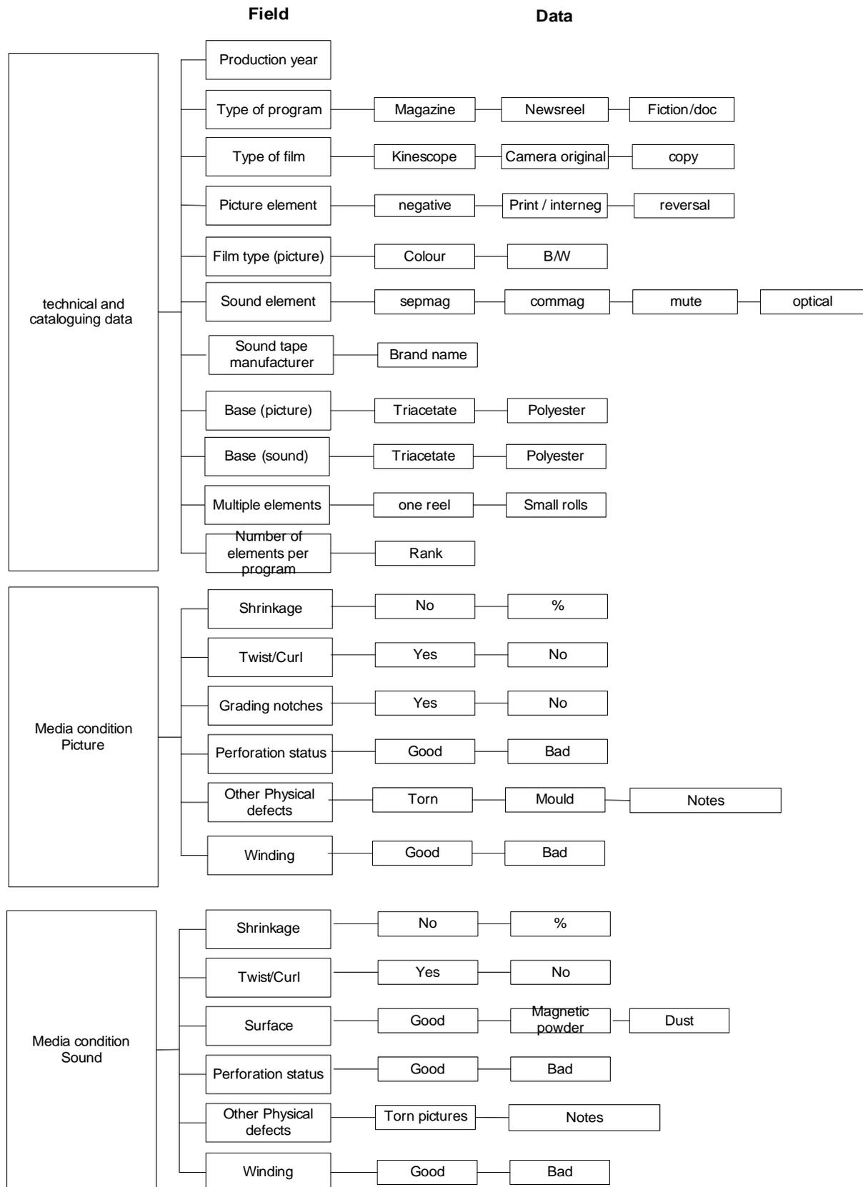
Figure 4-1: A database structure for films mapping and selection
