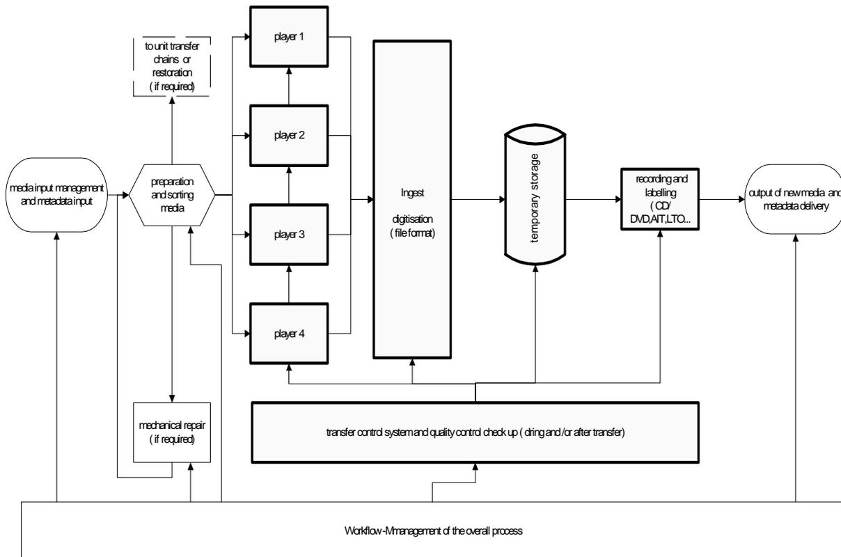
**Figure 4-9: A sample transfer chain composed of 4 parallel playbacks**
