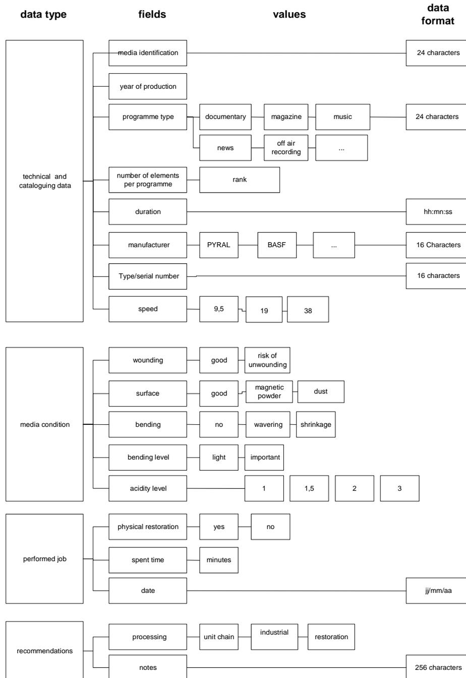
Figure 4-11 A database structure for 1/4" audio tapes mapping and selection
