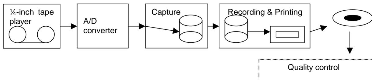
Figure 4-8: A conventional transfer chain for 1/4 Inch audio tapes
