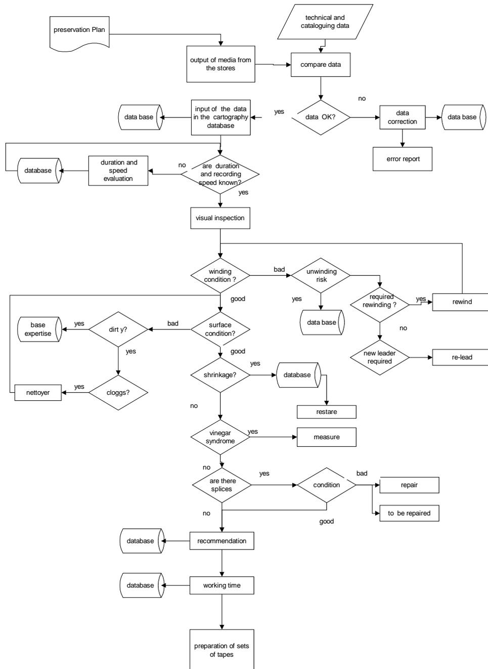
Figure 4-12: Mapping and Triage of 1/4" audio tapes
