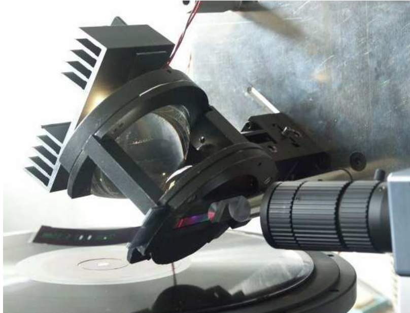
Figure 4 : A Closer view of the Condenser
