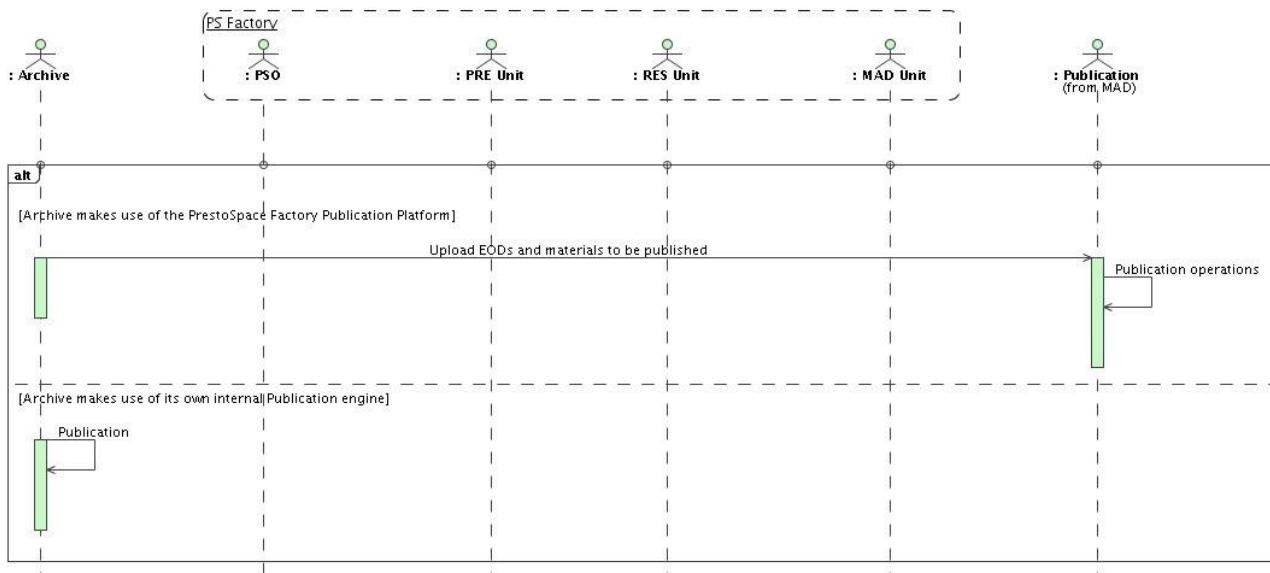
Figure 6-8 Sequence diagram representing the publication of EODs use case
