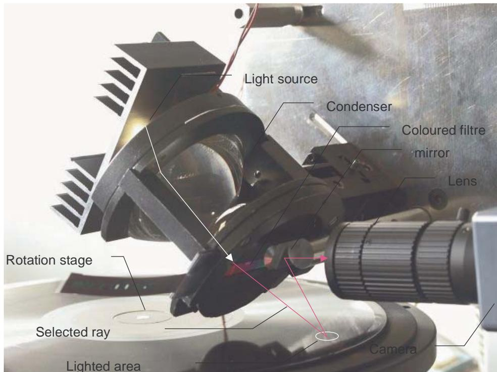
Figure 2 : The acquisition device for Figure 1
